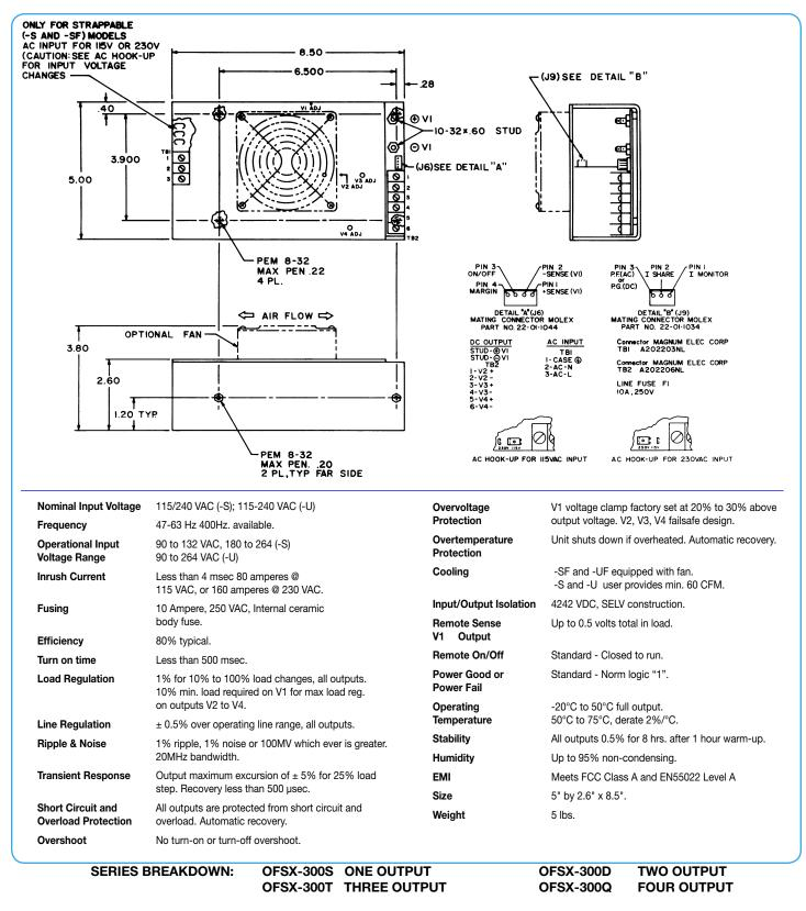
THEN ADD: -S FOR SELECTABLE INPUT OR -U FOR UNIVERSAL INPUT THEN ADD: F FOR FAN OR LEAVE OFF THE F IF THE USER WILL PROVIDE COOLING
