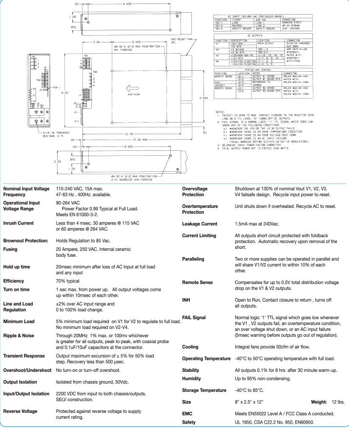
SERIES BREAKDOWN: GNX-1000X1-P where X1= S for Single output, D for Dual output, T for Triple output or Q for Quad output
