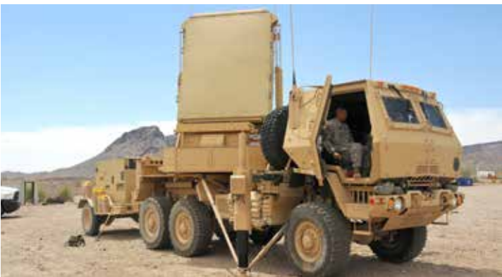
US Army AN/TPQ-53 Counterfire Radar
